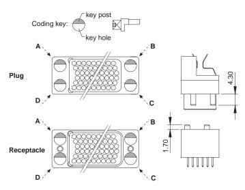
HARDWARE VARIATIONS The guides and the screw locking are supplied mounted: please consult the factory for order p/n and extraction tool.
