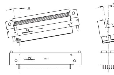
$\alpha$ =0°25' max, connectors equipped with one only dielectric inserts;  $\alpha$ =0°11' max, connectors equipped with two dielectric inserts;  $\alpha$ =0°07' max, connectors equipped with three dielectric inserts
