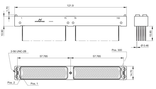
**RECEPTACLE CONNECTOR, 300 SOCKET CONTACTS,** WIRE WRAPPOST CONTACT TERMINAL STYLE
