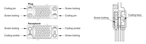
NOTE: the coding key is in thermoplastic polyester, the guide pin /socket and screw locking are in stainless steel
