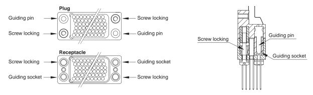
Connector supplied with two coding keys and two screw locking (only connectors without backpanel)
